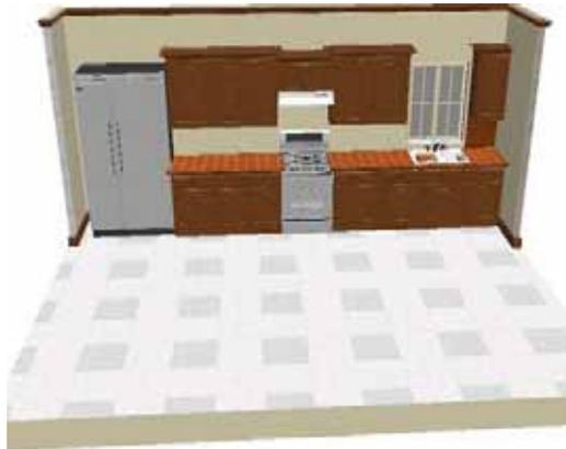
Fig. 8 Three Dimensional Drawing- Single Wall Shape Kitchen Layout
